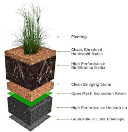
Focal Point biofiltration system. Credit: Convergent Water Tech
